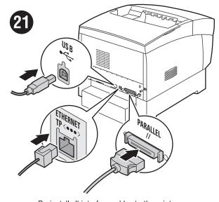
Re-install all interface cables to the printer. Print a Startup Page again. Check for defect to be eliminated. If defect is still found, repeat procedure from step 3 on.
