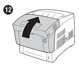
Close door A. Wait approx. 15 to 20 seconds. "Ready to Print" displays on the front panel when cleaning is complete.
