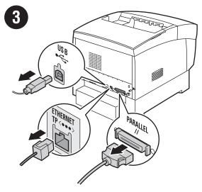
Remove all interface cables from the printer.
